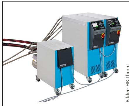
For variothermal temperature control HB-Therm employs two Thermo-5 temperature control units that are connected to the machine and mould via the Vario-5 switching unit.
