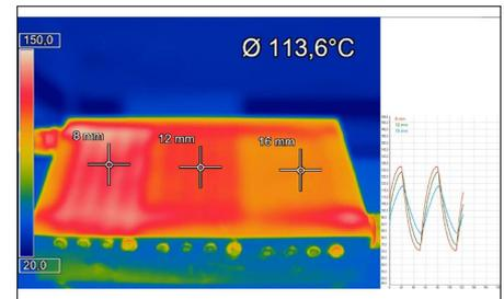
The infrared photograph shows a test mould. It shows the temperature pattern of a test plate with various temperature control channel distances.
